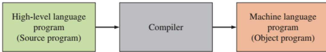
FIGURE 14-30 High-level to machine conversion with a compiler.
